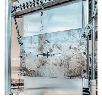
Static and dynamic panel tests of aircraft fuselage structures have been part of Applus+ IMA Dresden's portfolio for many years. This experience enables us to convert our testing machines, standardised fixtures as well as our optical measurement technology and high-speed camera systems to breadboard tests of aerospace structures in a short time.
