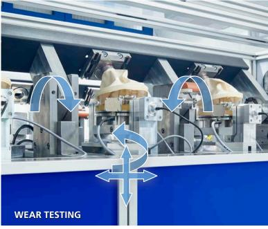
Joint implants are loaded for up to ten million cycles in the anatomically correct position under physiologic conditions in our laboratories. Thanks to the help of our accredited testing programs, we can simulate the lifetime of an implant.
