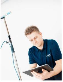
We check the noise characteristics of fittings and devices of water installations by measuring the valve noise level. For this purpose, the sound emitted by the valves is transmitted onto a measuring wall in our special testing laboratory, which records the airborne sound.
