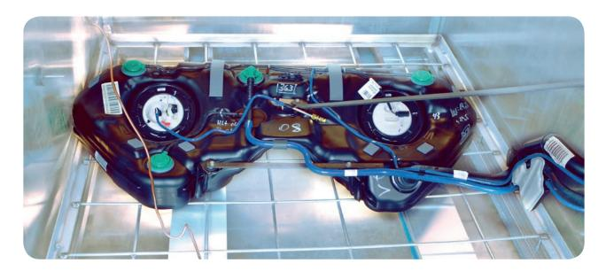
Fuels and lubricants damage the environment. That makes it all the more important that nothing should escape into the surroundings. In our laboratory, we test that not just the tank but also valves, fittings, interfaces etc. are strong, leak-proof and fully functioning.
